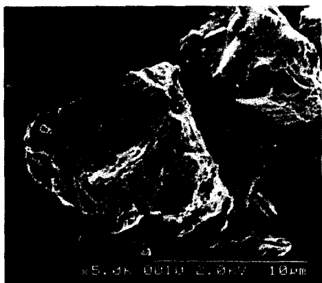
Fig. 4. SEM micrograph of core-shell particles obtained from green mesophase-pitch beads and phenol resins containing small amount of ground graphite.
